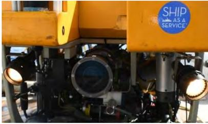
Figure 8 - Caméra principale (caisson) (source : SAAS)
